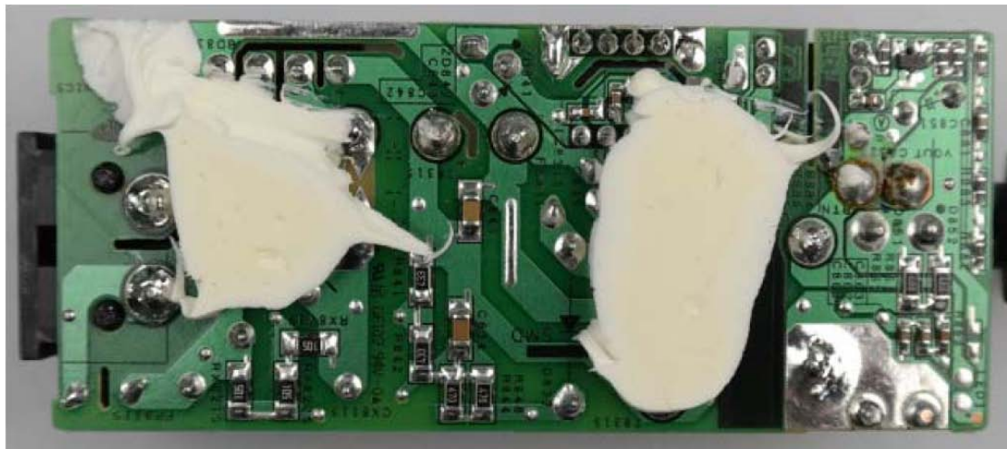
Before change A2514_DSM internal rear view
