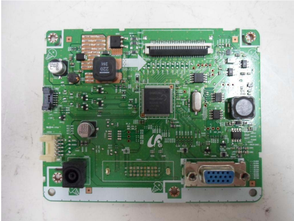
After change BN41-01967A (VGA) Internal front view
