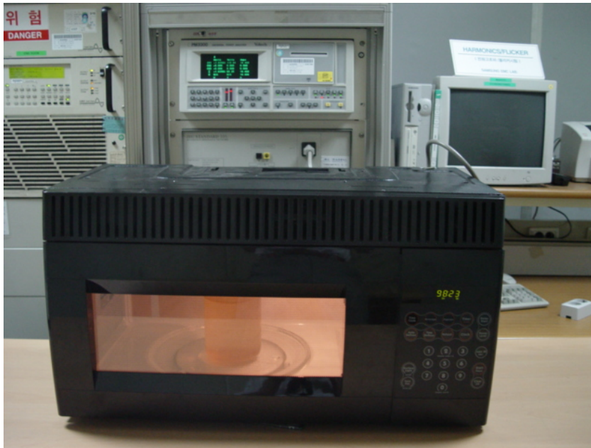
Fig.3 Test Setup for RF output power
