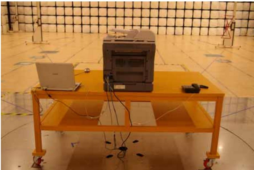
Picture 4. Radiated emission (Rear)
