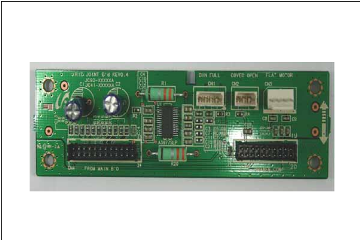
13) Top View of Joint B'D
