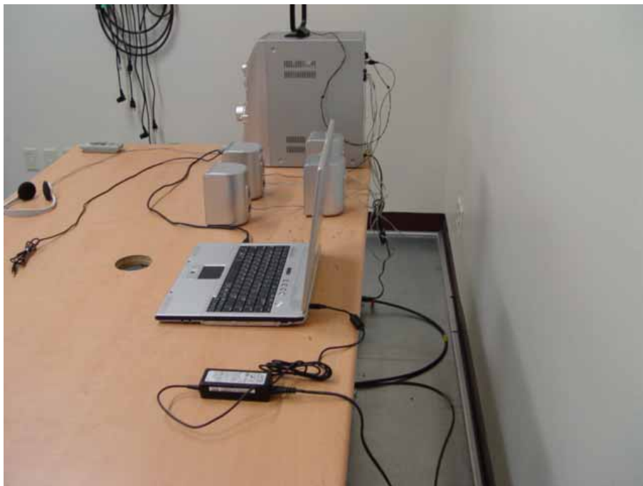
Picture 1. Conducted Emission(Side View)
