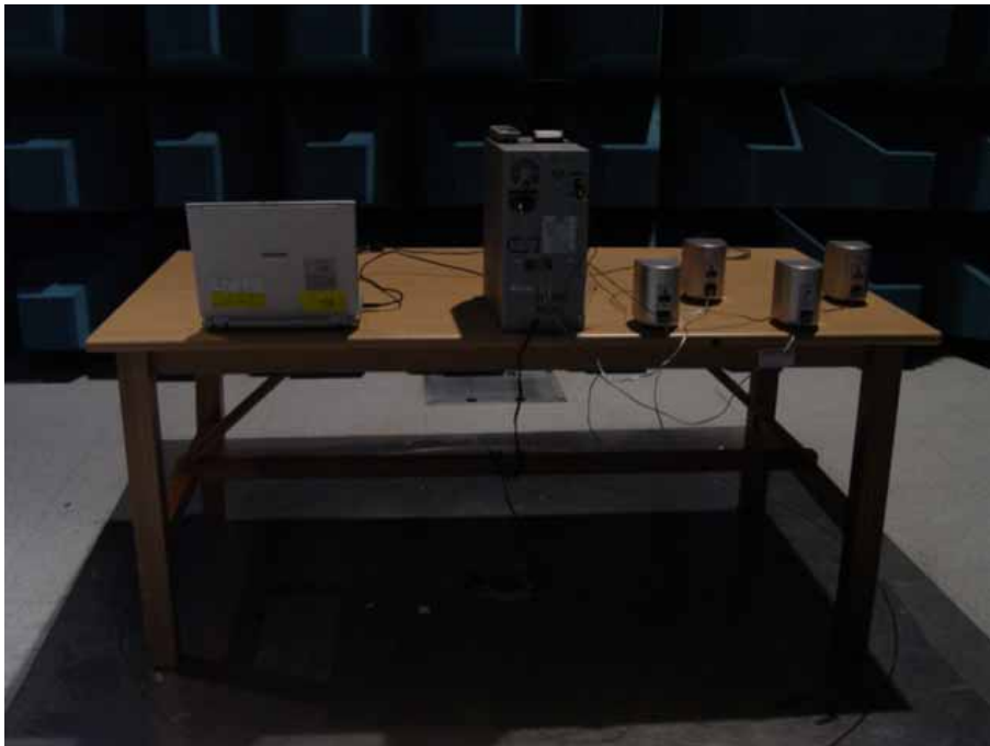
Picture 4. Radiated Emission (Rear View)
