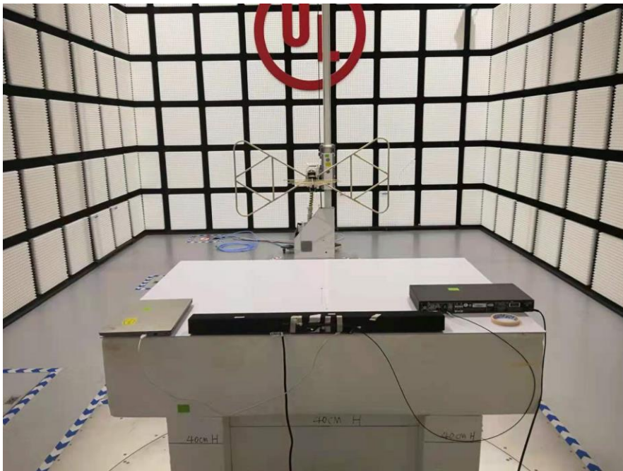
RADIATED RF MEASUREMENT SETUP (30MHz~1GHz)
