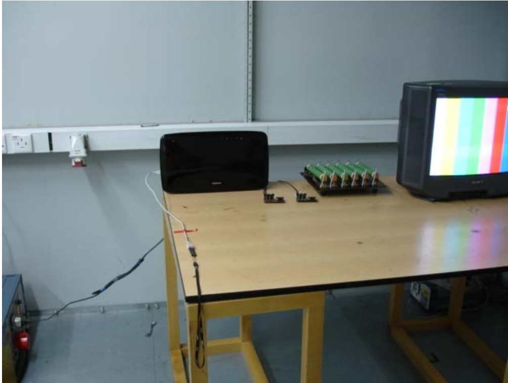
Photo 2 Antenna Terminal Voltage Disturbance Test
