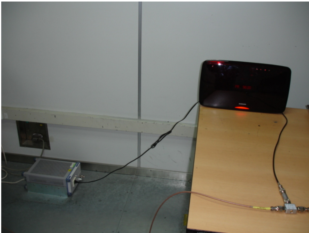
Photo 2 Antenna Terminal Voltage Disturbance Test
