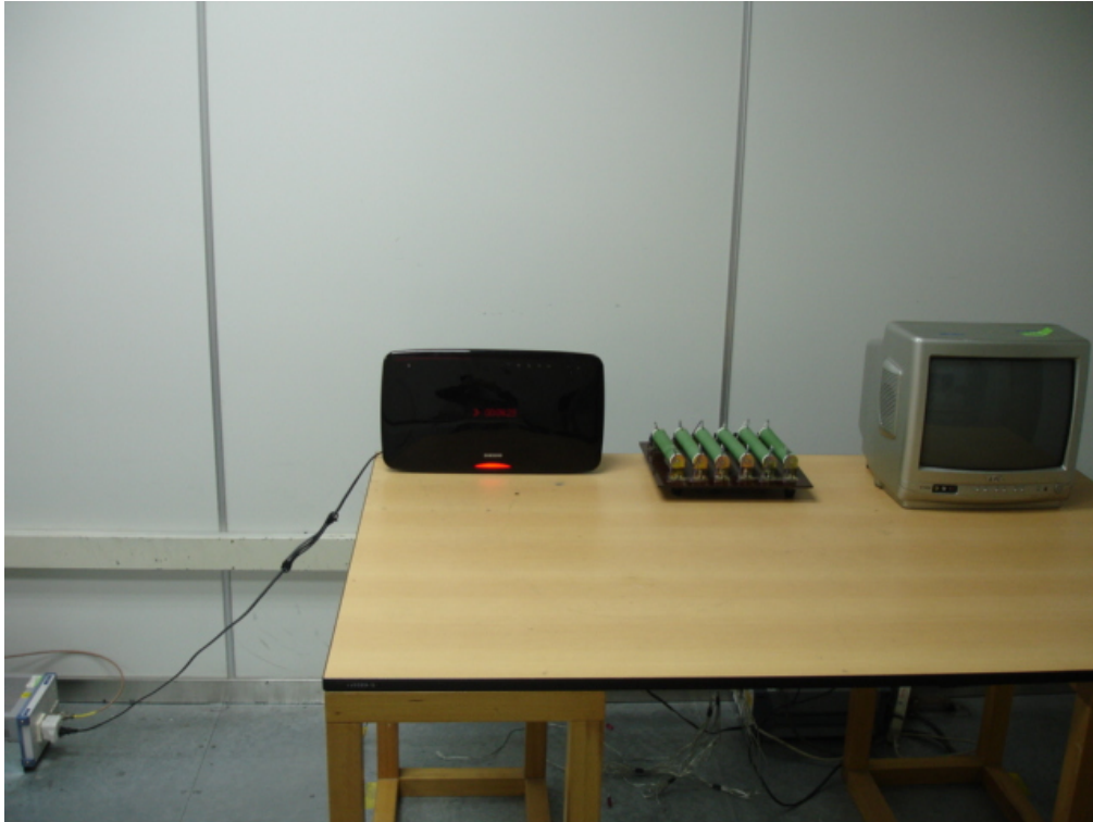
Photo 2 Antenna Terminal Voltage Disturbance Test
