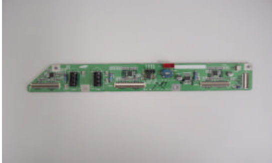
ADRESS BUFFER BOARD LJ TOP VIEW
