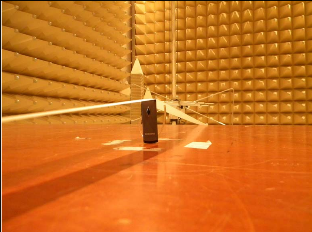
Photo of Field Strength & Spurious Emission Test
