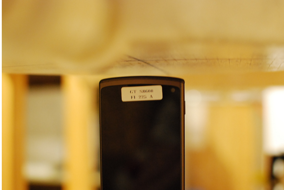
SAR Test Setup Photo 7: Top at 1.0 cm
