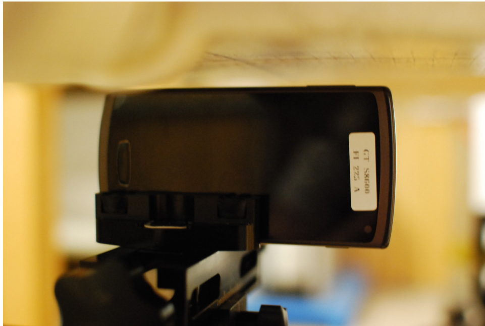
SAR Test Setup Photo 10: Left at 1.0 cm
