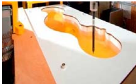
Figure 6-2 SAM Phantom with Simulating Tissue
