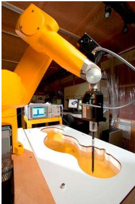
Figure 3-2 DASY4 SAR Measurement System
