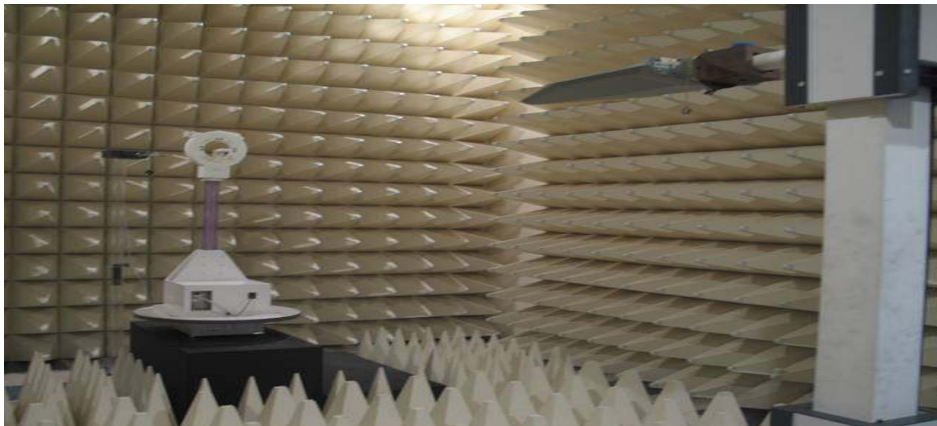
Figure2. Photograph of 3m Fully-Anechoic Chamber
