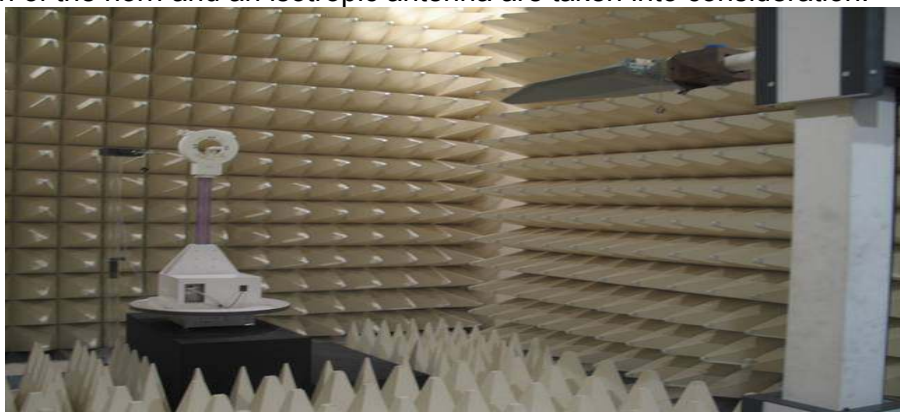
Figure2. Photograph of 3m Fully-Anechoic Chamber
