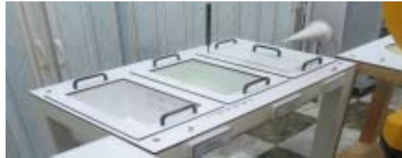
Figure 3.6 Modular Flat Phantom
