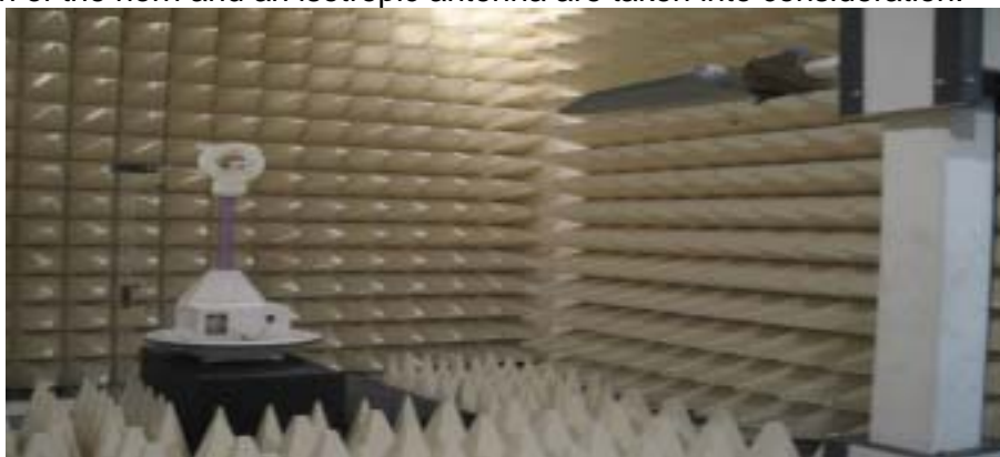
Figure2. Photograph of 3m Fully-Anechoic Chamber
