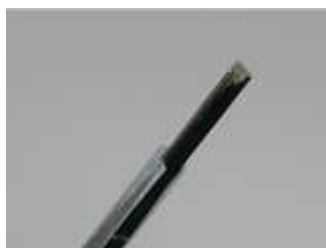
Figure 4.3 EX3DV4 E-field Probe
