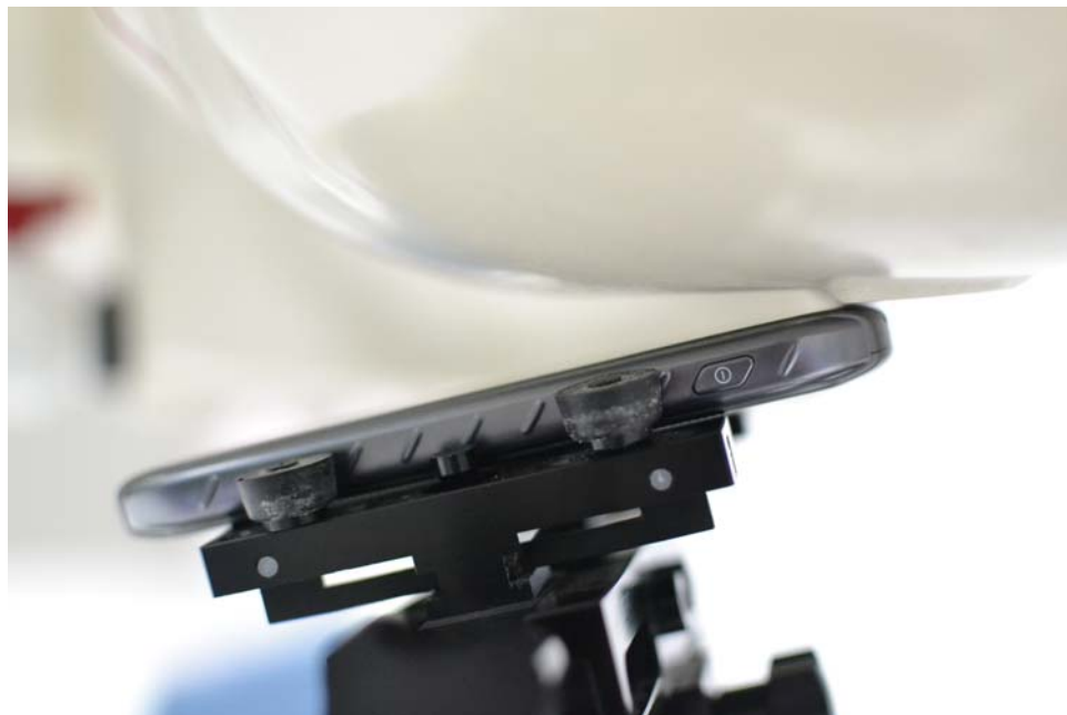
SAR Test Setup Photo 4 – Left Tilt
