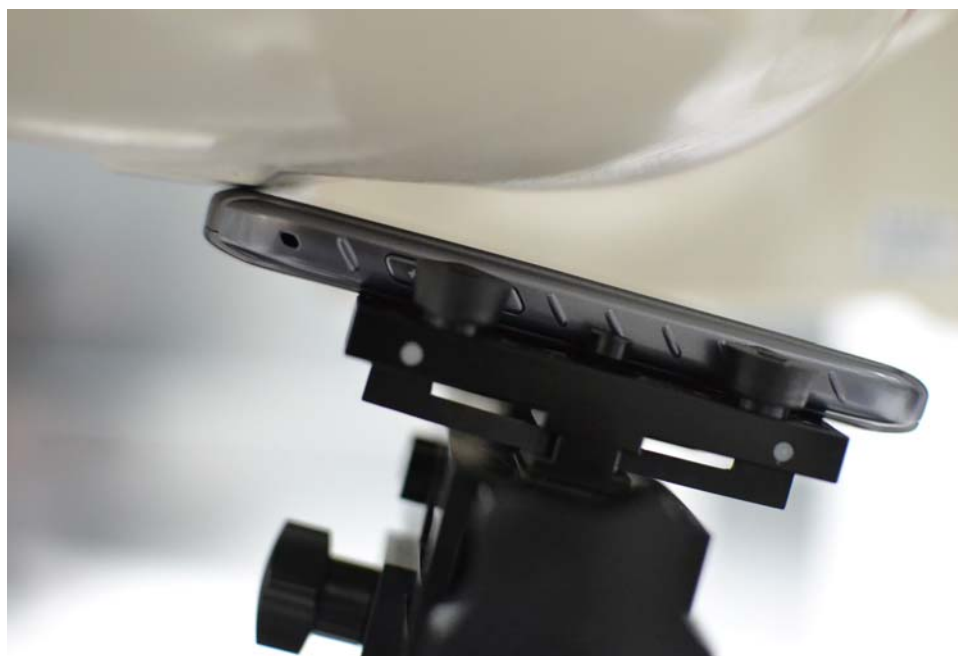
SAR Test Setup Photo 2 – Right Tilt
