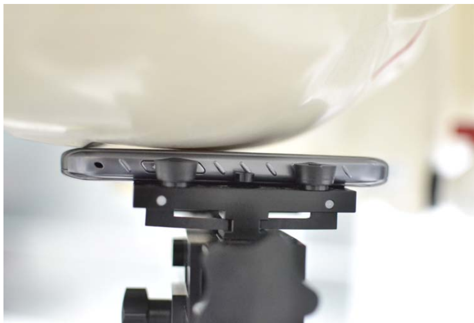
SAR Test Setup Photo 1 – Right Cheek
