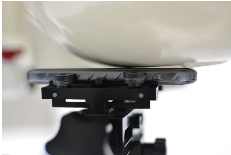
SAR Test Setup Photo 3 – Left Cheek
