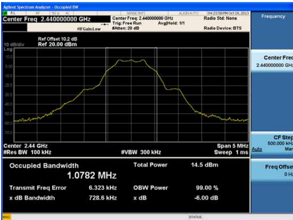
6dB Bandwidth plot (Mid-CH 19)
