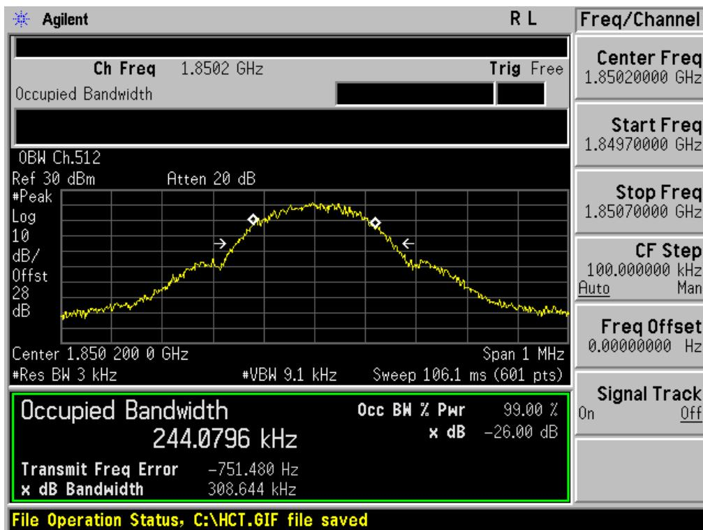
■ GSM1900 MODE (661 CH.) Occupied Bandwidth
