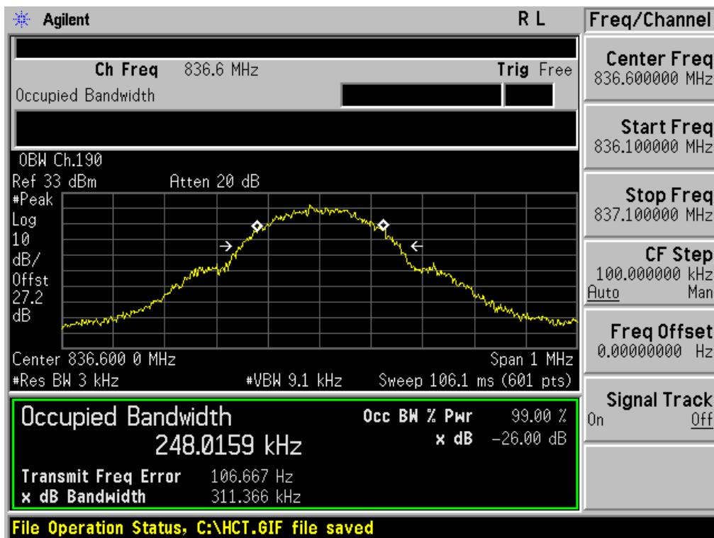
■ GSM850 MODE (251 CH.) Occupied Bandwidth
