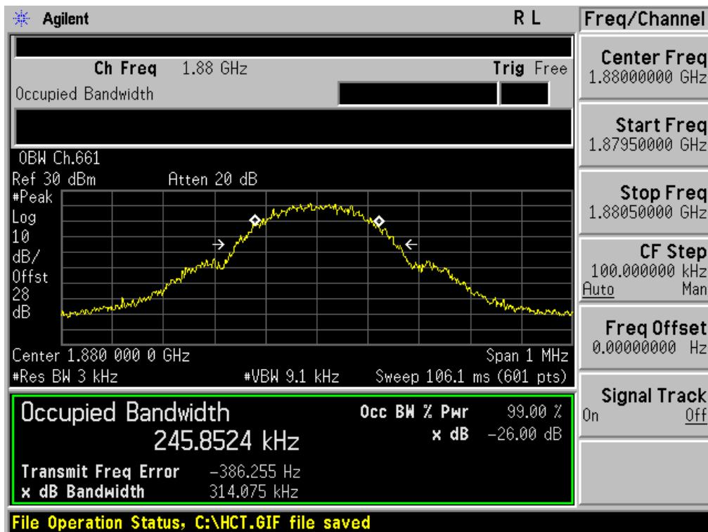
■ GSM1900 MODE (810 CH.) Occupied Bandwidth
