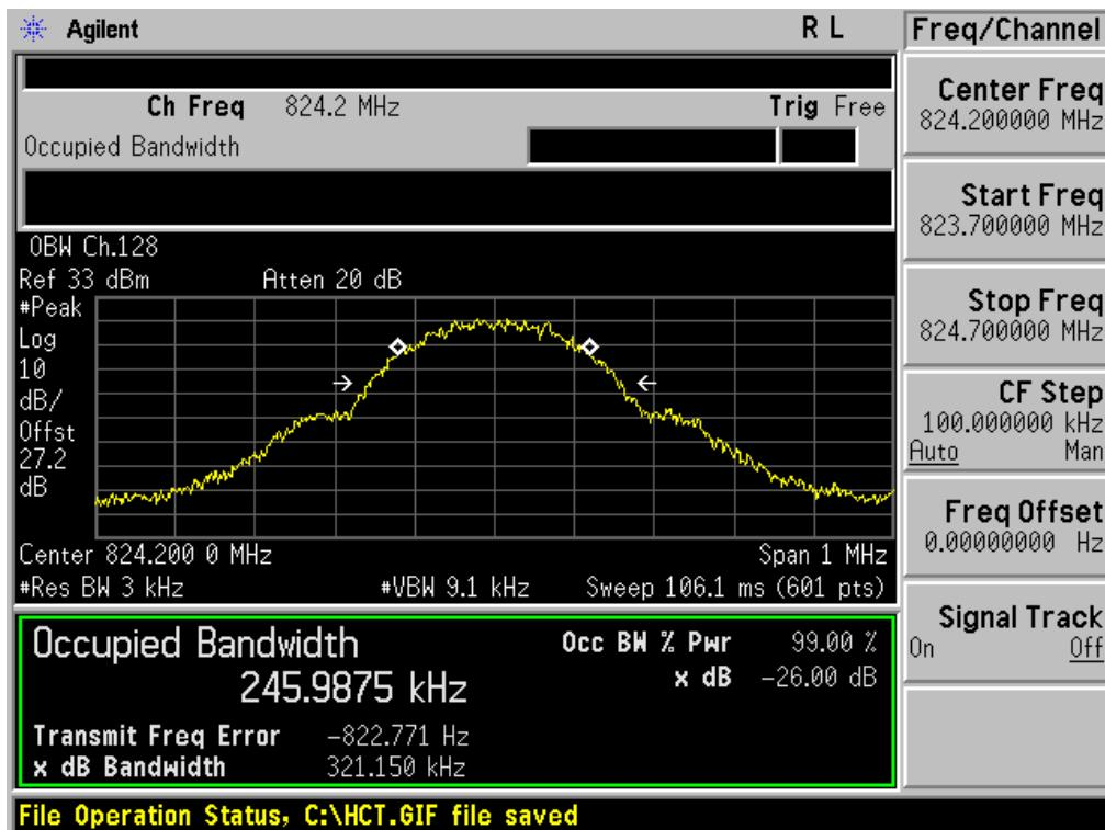
■ GSM850 MODE (190 CH.) Occupied Bandwidth
