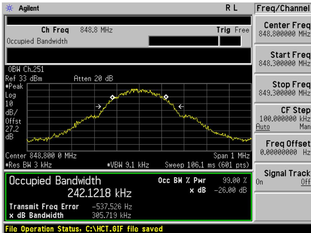
■ GSM1900 MODE (512 CH.) Occupied Bandwidth
