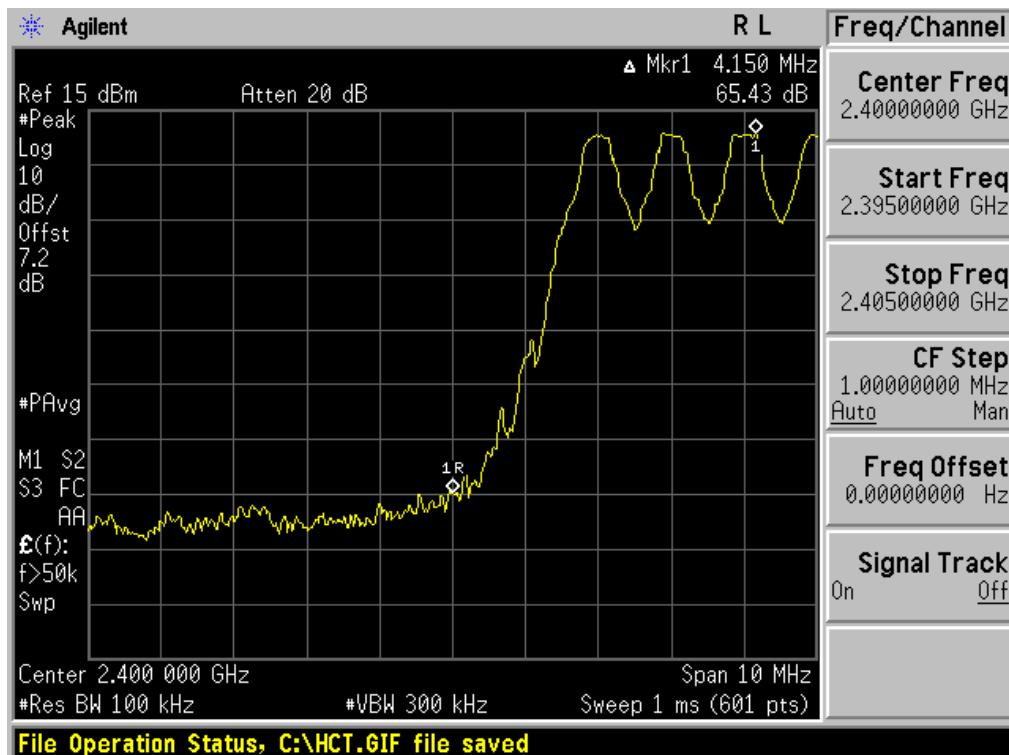
Test Plots with hopping (GFSK)
