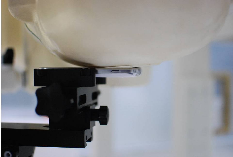
SAR Test Setup Photo 3 – Left Cheek
