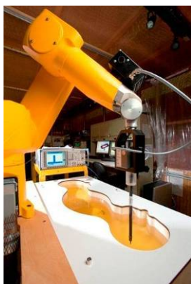
Figure 3-1 SAR Measurement System
