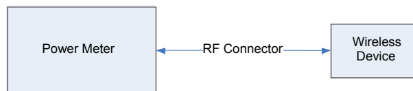
Figure 9-2 Power Measurement Setup
