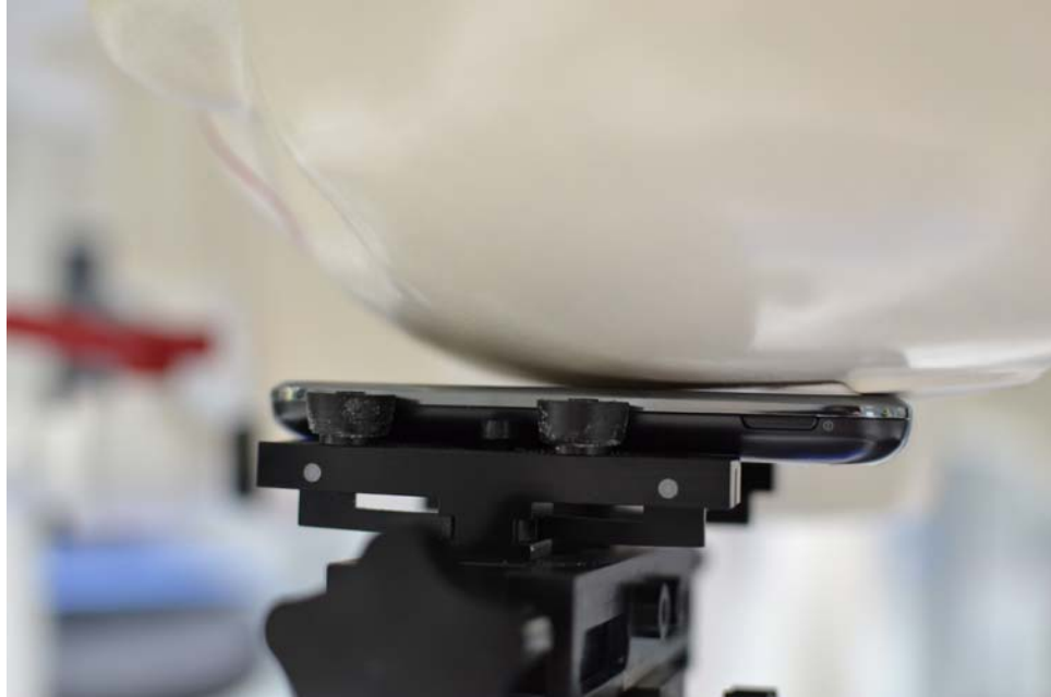
SAR Test Setup Photo 3 – Left Touch
