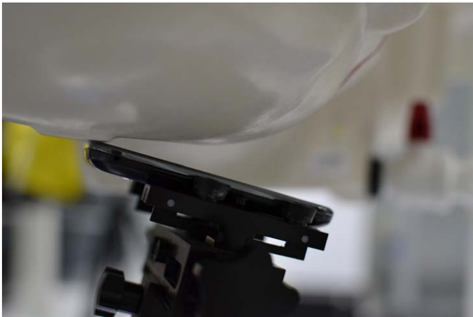
SAR Test Setup Photo 2 – Right Tilt
