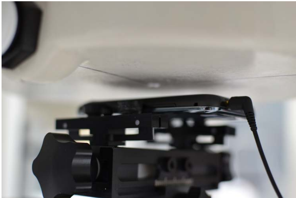
SAR Test Setup Photo 10 – Back Side Body-worn at 1.0 cm
