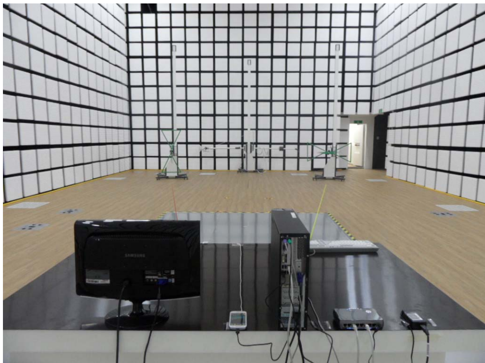
[ Radiated Disturbance for Below 1 GHz – Rear ]
