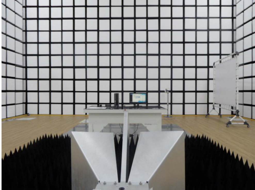
[ Radiated Disturbance for Above 1 GHz – Front ]
