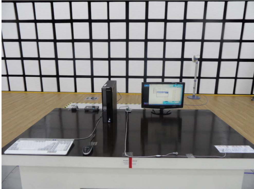
[ Radiated Disturbance for Below 1 GHz – Front ]
