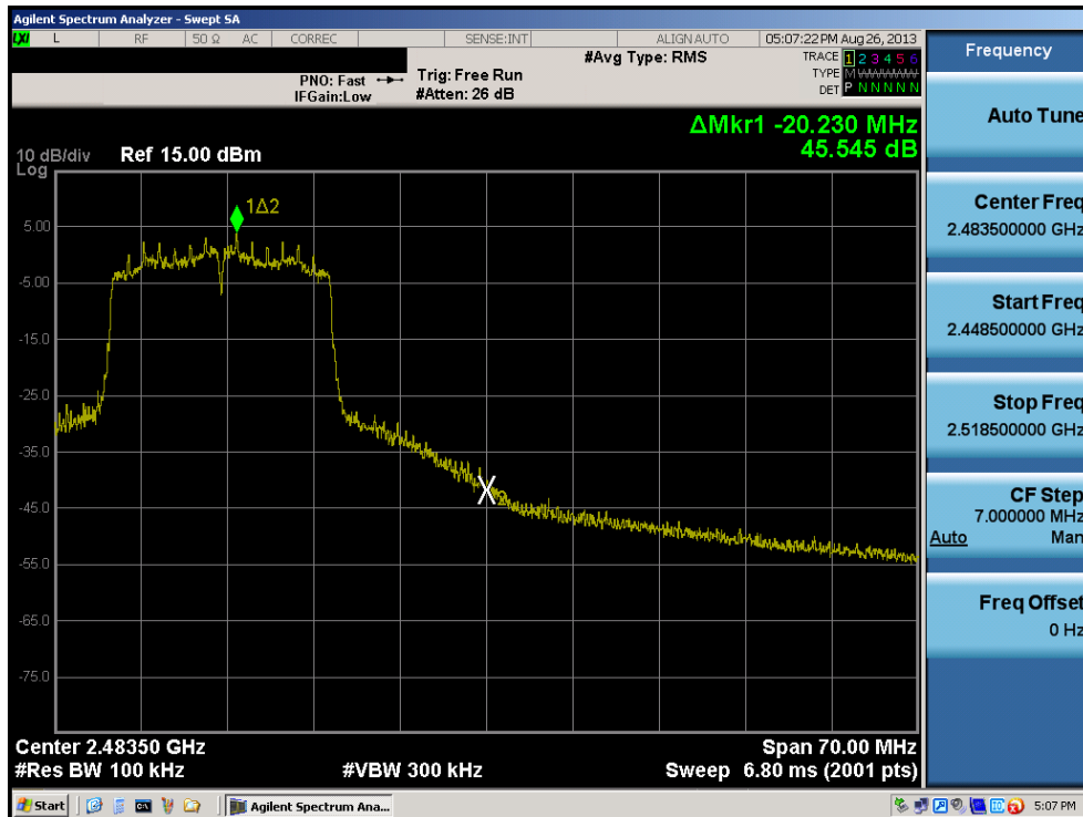
Plot 6-24. Band Edge Plot (802.11n (2.4GHz) – Ch. 11)
