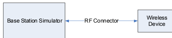
Figure 8-1 Power Measurement Setup
