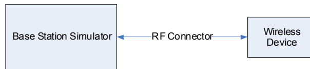
Figure 8-2 Power Measurement Setup
