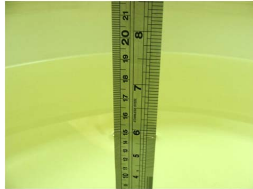
Fig 6.2 Photo of Liquid Height for Body SAR
