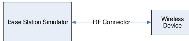
Figure 8-1 Power Measurement Setup
