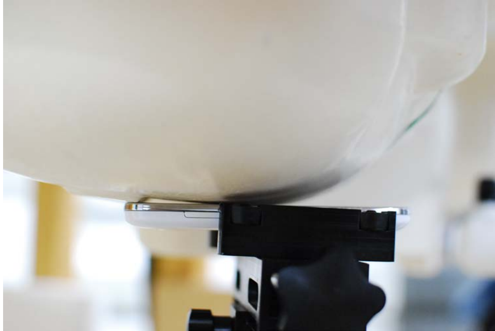
SAR Test Setup Photo 1: Right Cheek
