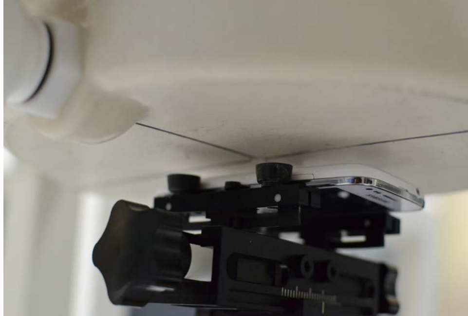
SAR Test Setup Photo 5: Back at 1.0 cm
