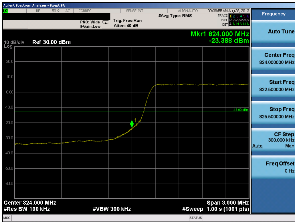
Plot 8-15. Lower Band Edge Plot (5.0MHz QPSK – RB Size 25)
