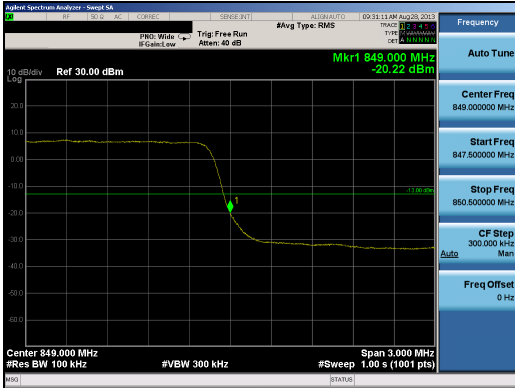
Plot 8-14. Upper Band Edge Plot (3.0MHz QPSK – RB Size 15)
