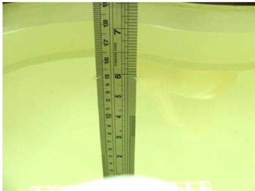
Fig 6.1 Photo of Liquid Height for Head SAR
