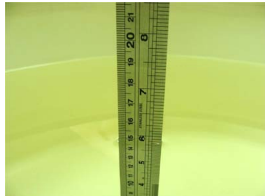
Fig 6.2 Photo of Liquid Height for Body SAR
