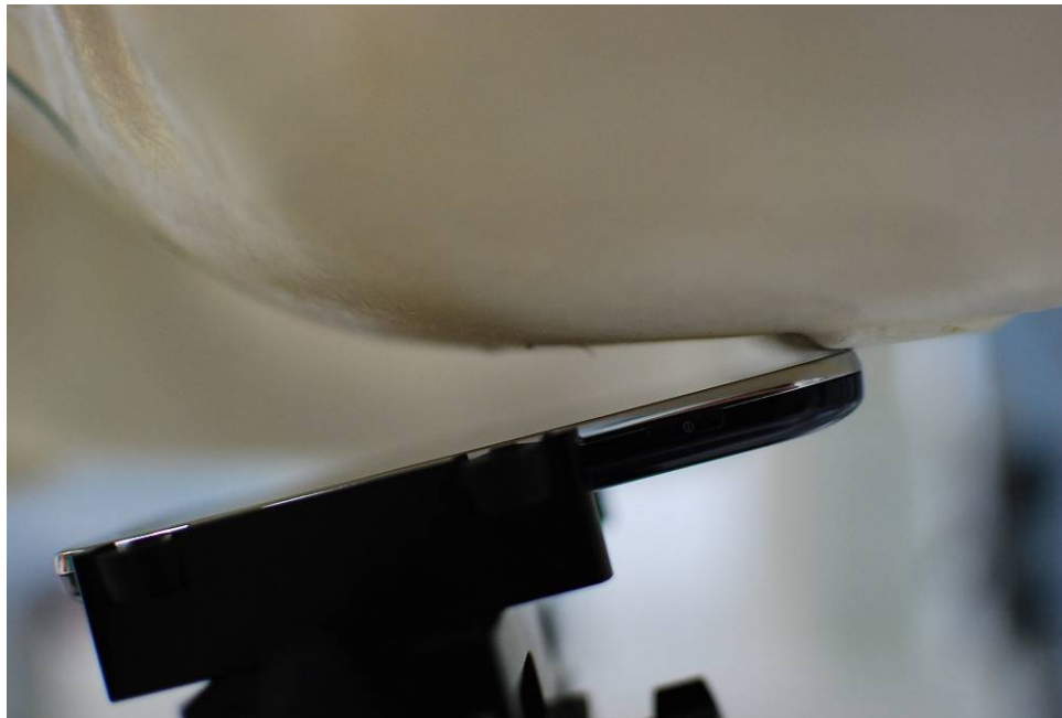
SAR Test Setup Photo 4 – Left Tilt
