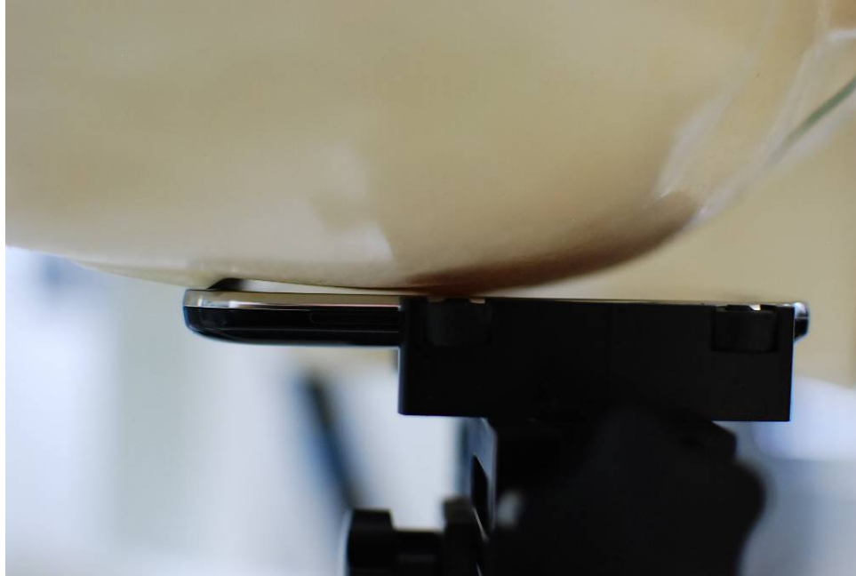
SAR Test Setup Photo 1 – Right Cheek
