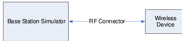
Figure 11-1 Power Measurement Setup
