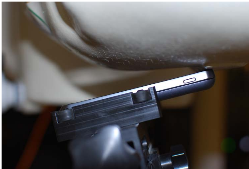
Figure 20-4 SAR Test Setup Photo 4
