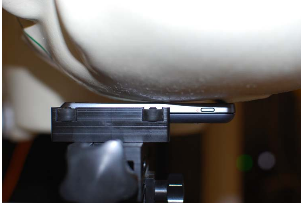
Figure 20-3 SAR Test Setup Photo 3
