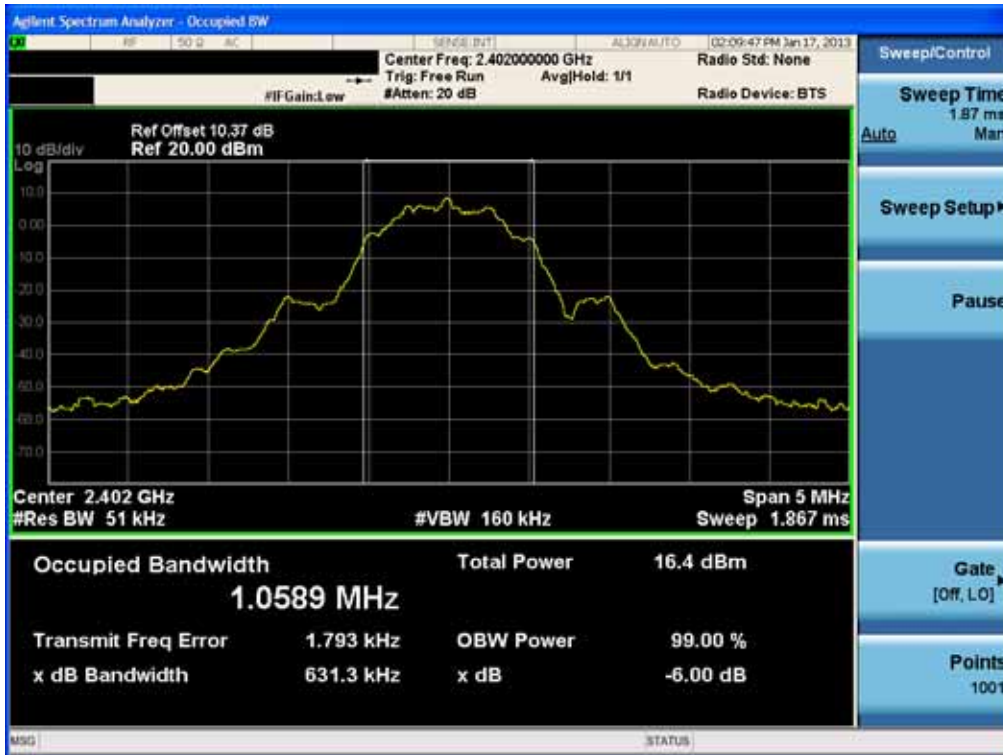
6dB Bandwidth plot (Low-CH 0)
