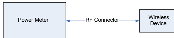
Figure 8-2 Power Measurement Setup
