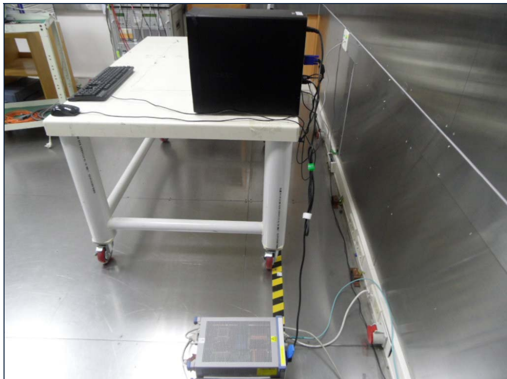
[ Conducted Disturbance – Rear ]
