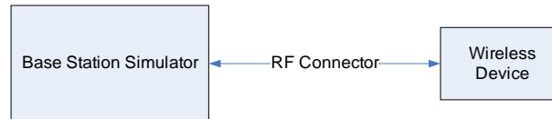
Figure 8-2 Power Measurement Setup
