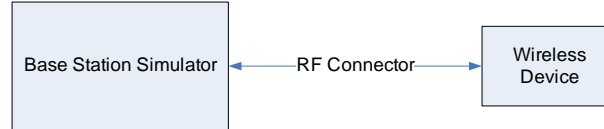
Figure 8-2 Power Measurement Setup
