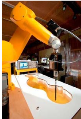
Figure 3-1 SAR Measurement System
