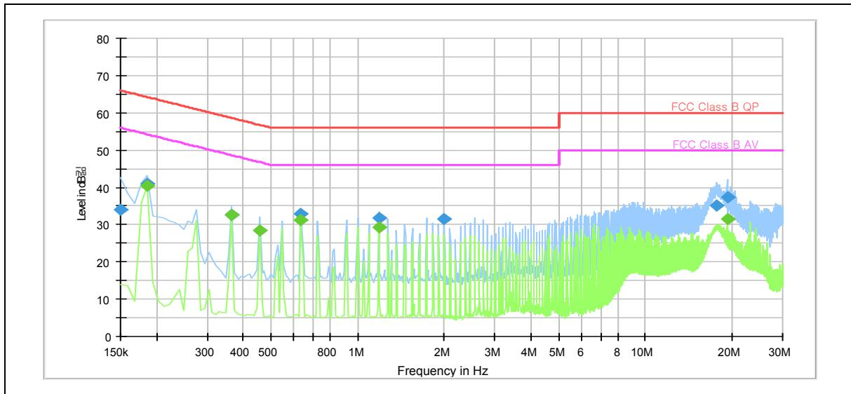
Note 1) Two graphs measured for both Live(L1) and Neutral(N) of the LISN are combined into one graph.
