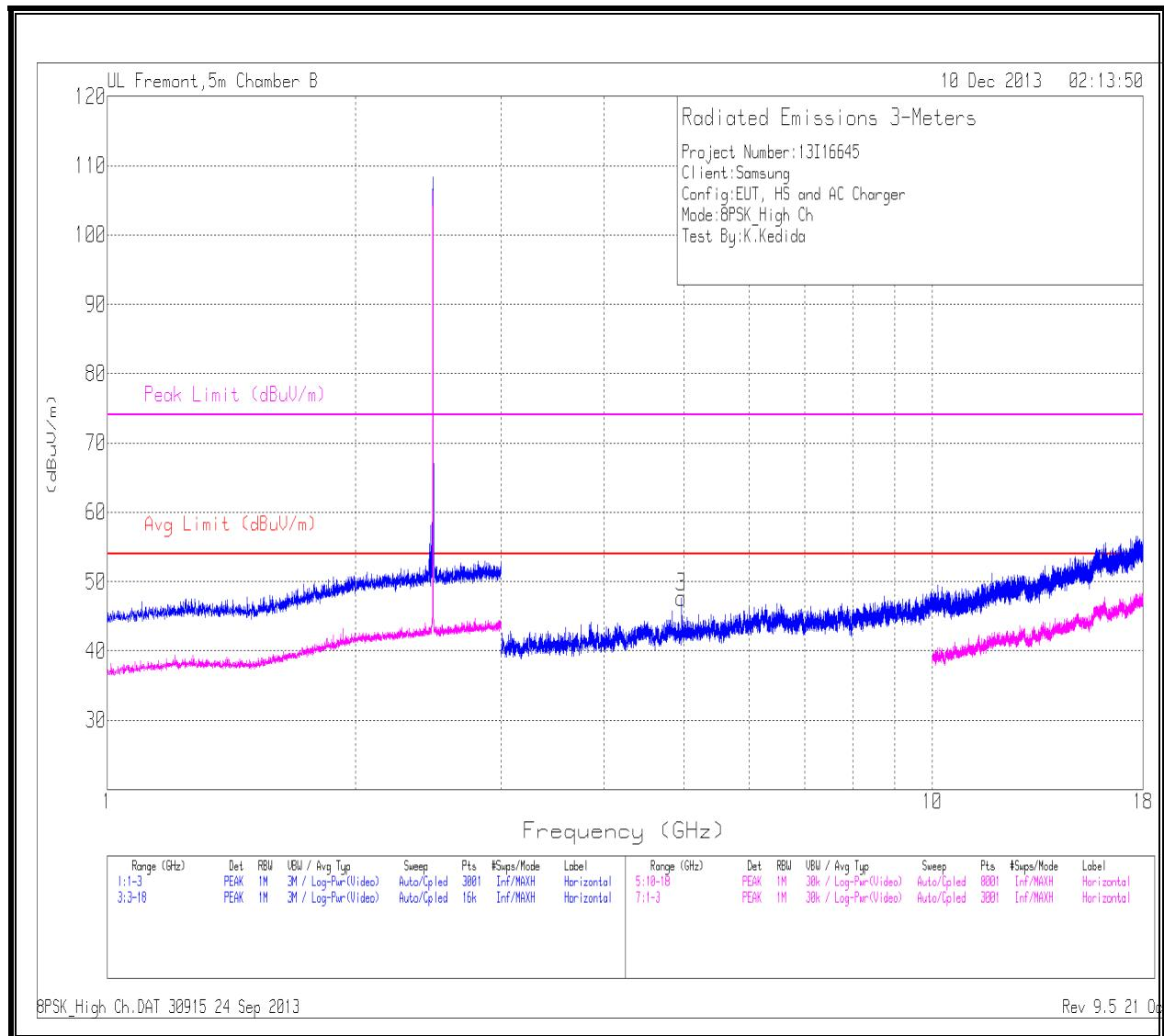
Note: Emission was scanned up to 26GHz; No emissions were detected above the noise floor which was at least 20dB below the specification limit.
