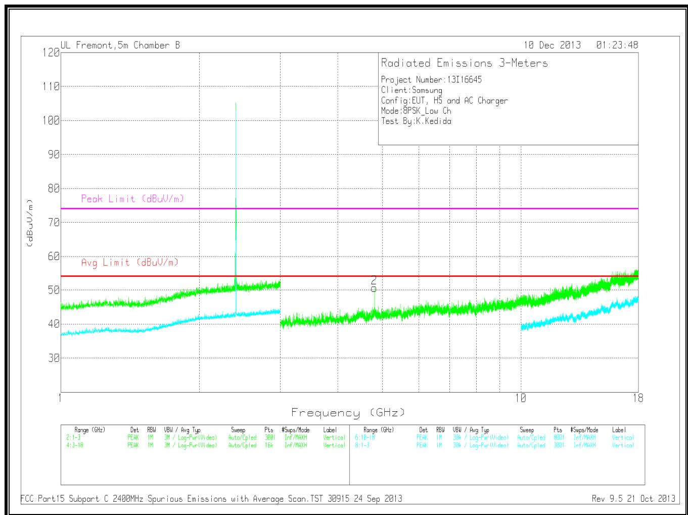
Note: Emission was scanned up to 26GHz; No emissions were detected above the noise floor which was at least 20dB below the specification limit.
