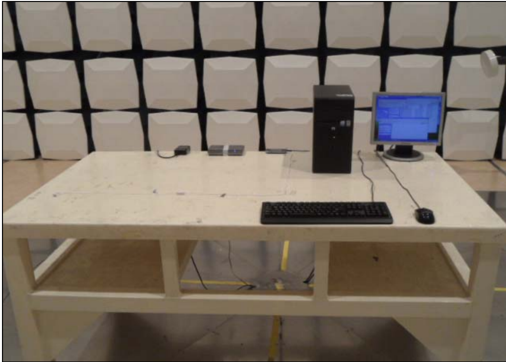
[ Radiated Disturbance for Below 1 GHz – Front ]
