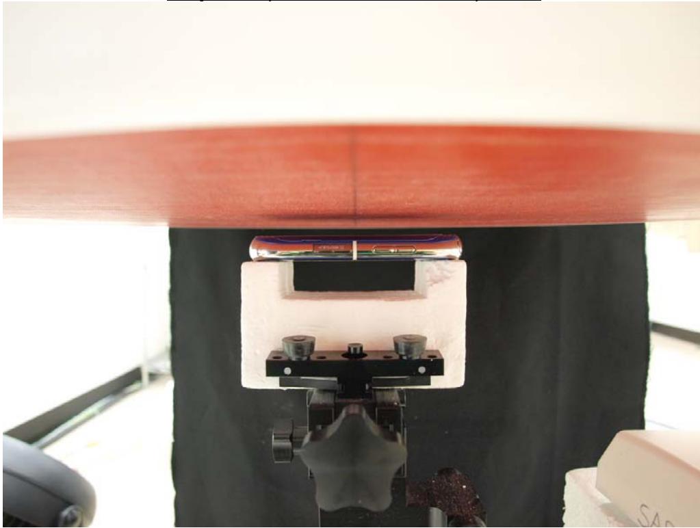
Body - Rear with 10 mm Separation (with Headset)
