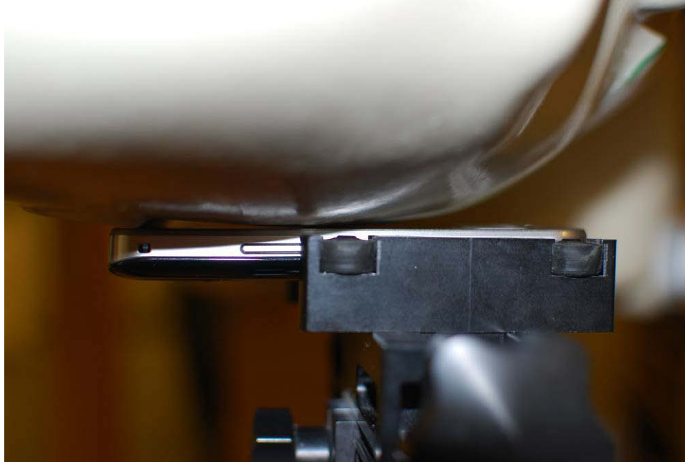
Figure 21-1 SAR Test Setup Photo – Right Touch
