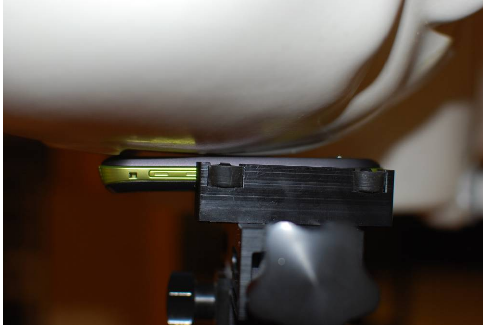
Figure 21-1 SAR Test Setup Photo 1
